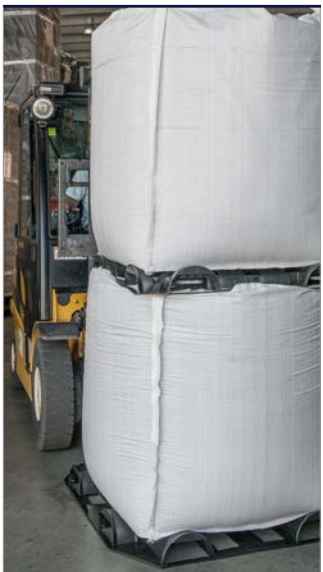
Units can be separated again easily and without damage by forklift tines.
